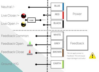
Failsafe versions have internal capacitor, this is charged whilst power is applied. When power is removed, the actuator will close or open depending on what you have ordered. Re-apply power and the capacitor will charge again and is always being charged when power is applied. When actuator is powered, heater is working.
